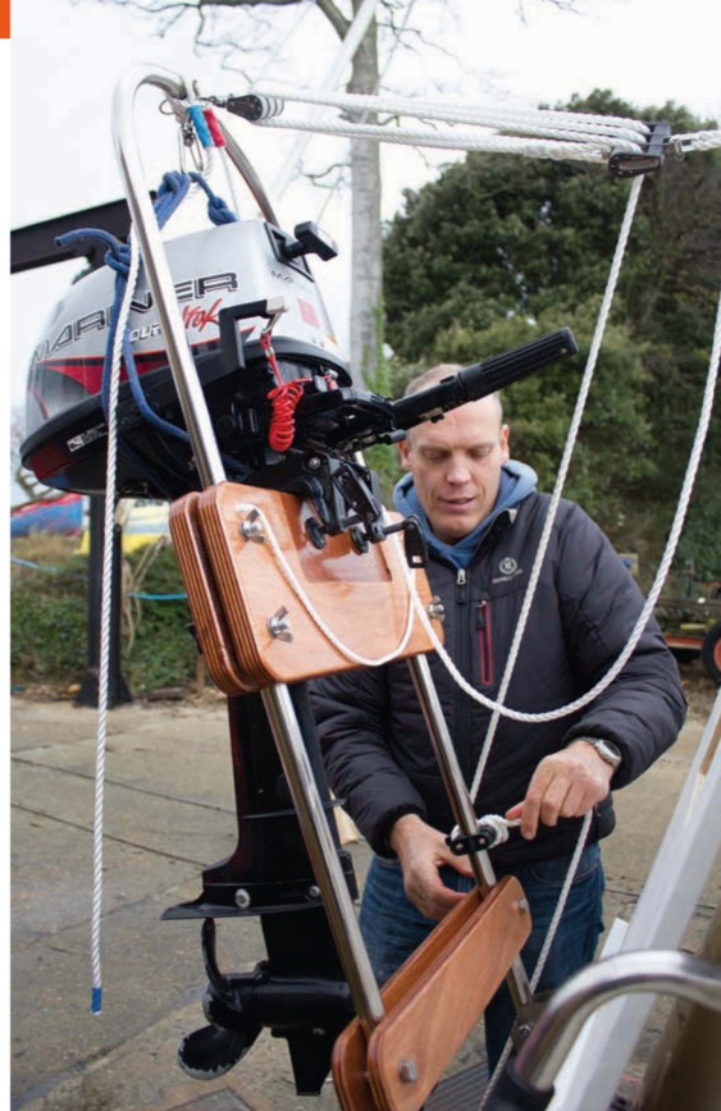
Above: The system involves a few lines which need carefully managing Left: The outboard also requires its own lifting sling
